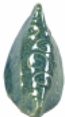
GLW12 over GLW31 Dry Rust
